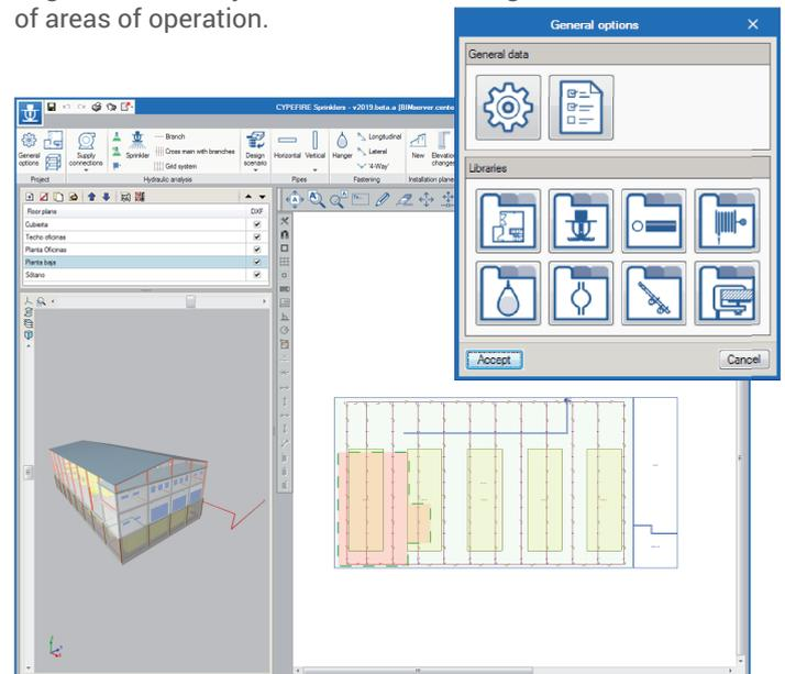
The users can see and easily correct the errors on the main elements of the model after the analysis (tank, pipes, sprinklers, pumps).
